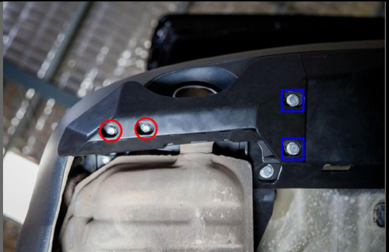
The WK2 Rear Bumper Guard (Corner Protection Kit) is now fully installed.
